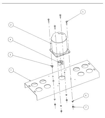
Fig. 3 Motor Base Assembly
